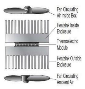
Fig-1: Schematic construction of Thermoelectric AC
